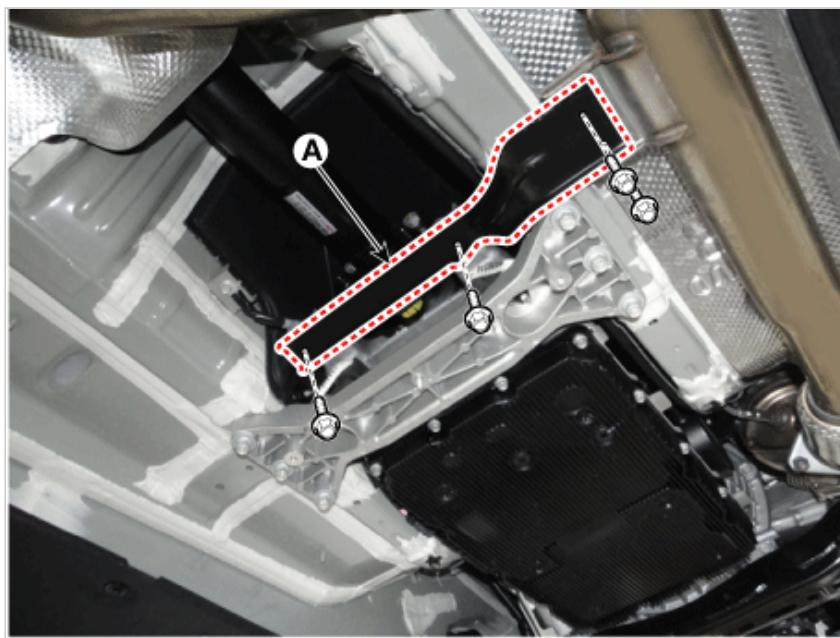
4. Remove the front propeller shaft (A).
